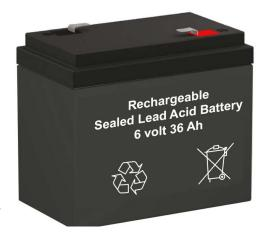
These rechargeable batteries are lead-lead dioxide systems. The dilute sulfuric acid electrolyte is absorbed by separators and thus immobilized. Should the battery be accidentally overcharged producing hydrogen and oxygen, special one-way valves allow the gases to escape thus avoiding excessive pressure build-up. Otherwise, the battery is completely sealed and is, therefore, maintenance-free, leak proof and usable in any position.
