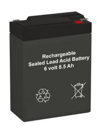
These rechargeable batteries are lead-lead dioxide systems. The dilute sulfuric acid electrolyte is absorbed by separators and thus immobilized. Should the battery be accidentally overcharged producing hydrogen and oxygen, special one-way valves allow the gases to escape thus avoiding excessive pressure build-up. Otherwise, the battery is completely sealed and is, therefore, maintenance-free, leak proof and usable in any position.
